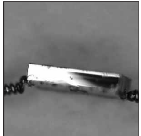
.003" Wire Welded to .003" Platinum
