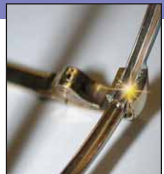
Frame Repair - Front to End Piece
